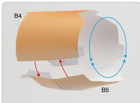
④ Assemble B1, B2 and B3, and B4 and B5.
