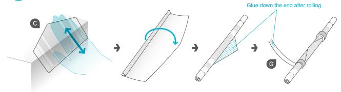
Add curves by pressing and rolling it against the corner of a table, with the printed side face up.
