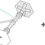
Tie one end of the band to the band stopper, and the other end to the middle of the axle.
