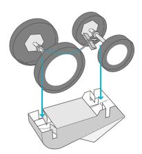
Fit the axles into the grooves of the body. Check that the wheels spin smoothly.
