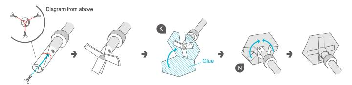
Cut three, equally-spaced slots in both ends of part C, up to the red valley fold line, and bend them back.
