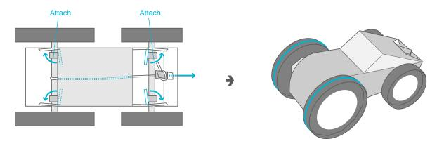
Pull the band stopper through the hole in part A. Be careful that the band doesn't come undone.
