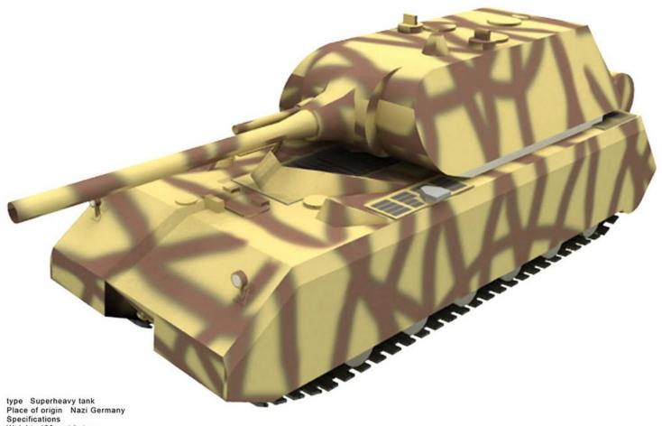
Weight 192 metric tons Length 10.09 m (33 ft) Width 3.67 m (12 ft) Height 3.63 m (11.9 ft)
