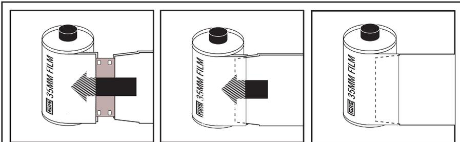
Light-safety is created by sandwiching the film between two layers of cardboard, and inserting those layers into the already light safe film canister. Carefully slide both tabs into the film canister, taking care to push the canister snugly against the frame.
