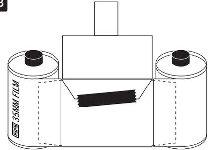
After sliding the cardboard tabs into the film canisters, wrap the top of the box over the back and tape it down. This should secure the entire box.
