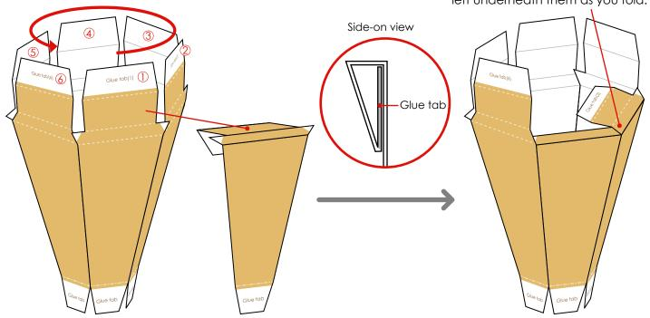
For glue tab (6), tuck the white triangles on the tabs on both sides underneath it as you fold.
