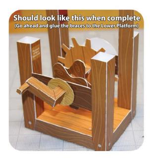
Glue Crank Shaft RearCap to the end of Crank Shaft.
